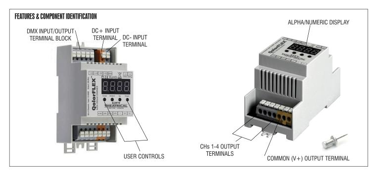
The QolorFLEX 4x5A DINrail Dimmer can control a full 20A of LED tape spread over four channels of 5A each. It uses constant voltage technology which ensures consistent full range dimming that is especially important at low end light levels. The unit mounts to a standard hat section DINrail, and has terminal blocks for all electrical and data connections.
